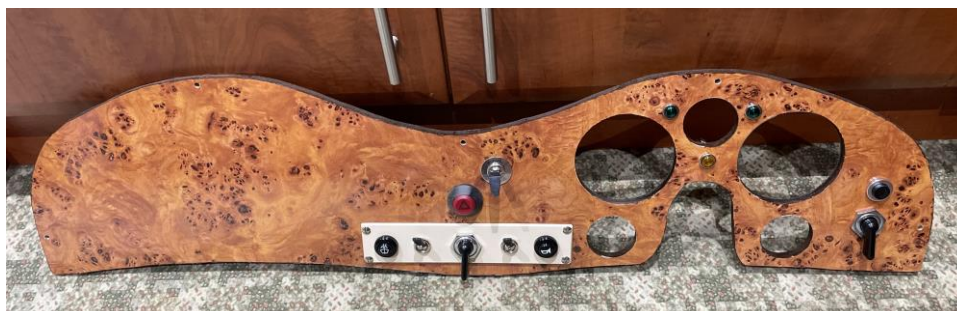
The completed switches and warning lights.
